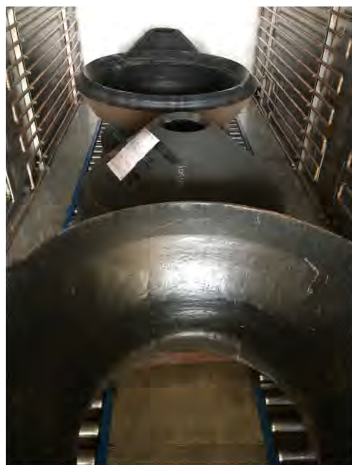
Figure 6. 14,000 lbs of Mn crusher cone mantles in the 36K
