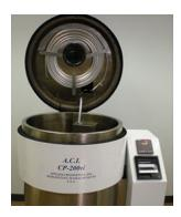
Items are slowly cooled over several days to -320° F using nitrogen gas in a specially designed tank and then returned to room temperature. DCT is a permanent, through-material process that doesn't erode like surface coatings.
