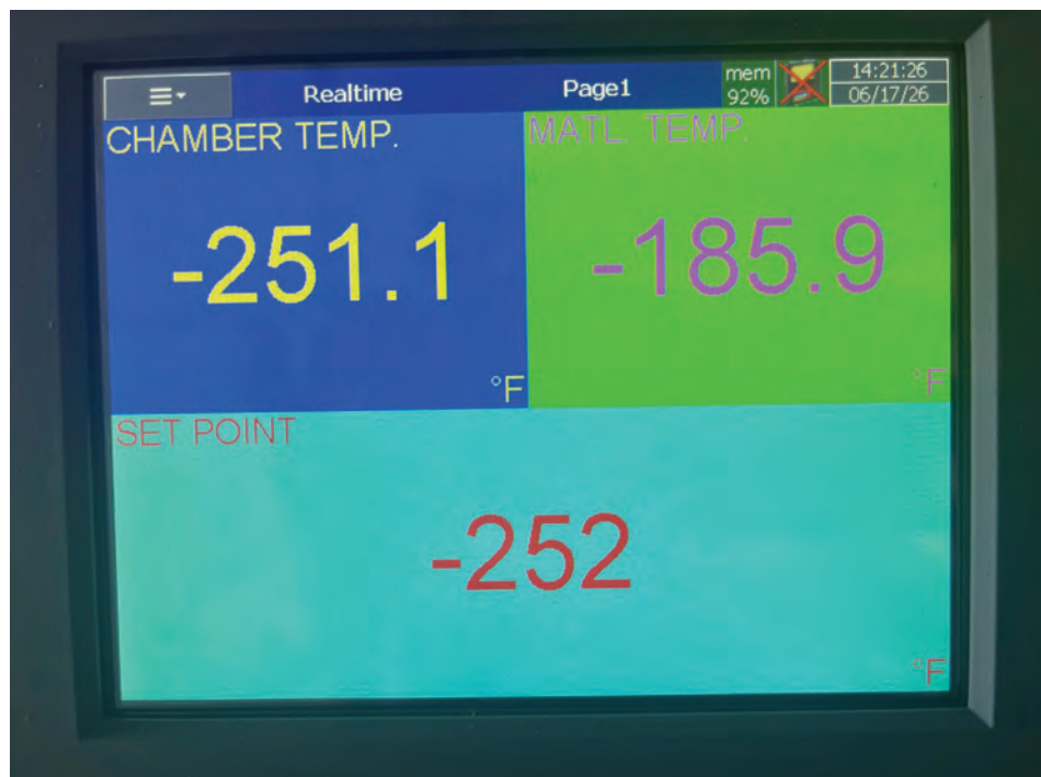
Figure 1. Chamber vs material temp - 10,000 lb payload on the way -294 °F. Credit: J. Cahn
