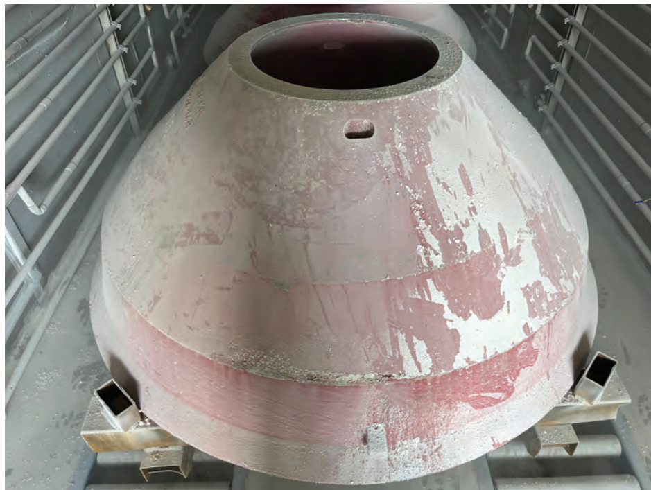
Figure 2. Slow cooling a 14,000 crusher liner payload. Credit: J. Cahn
