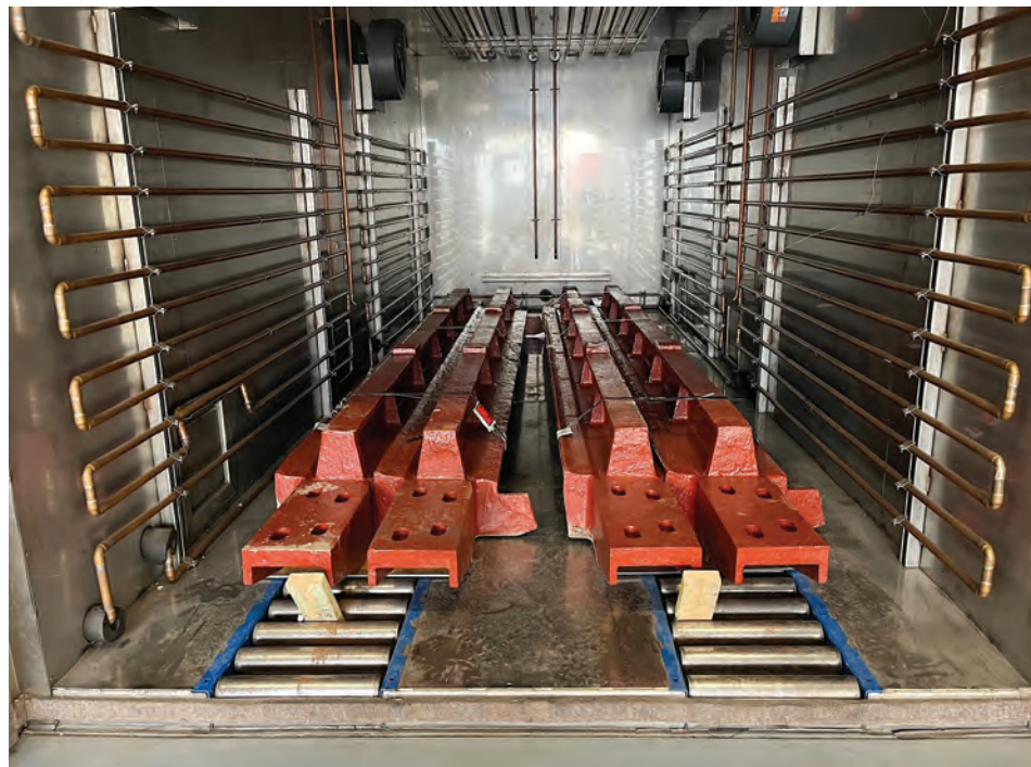
9,200 pounds of manganese steel feeder pans undergoing DCT. Credit: Jack Cahn
